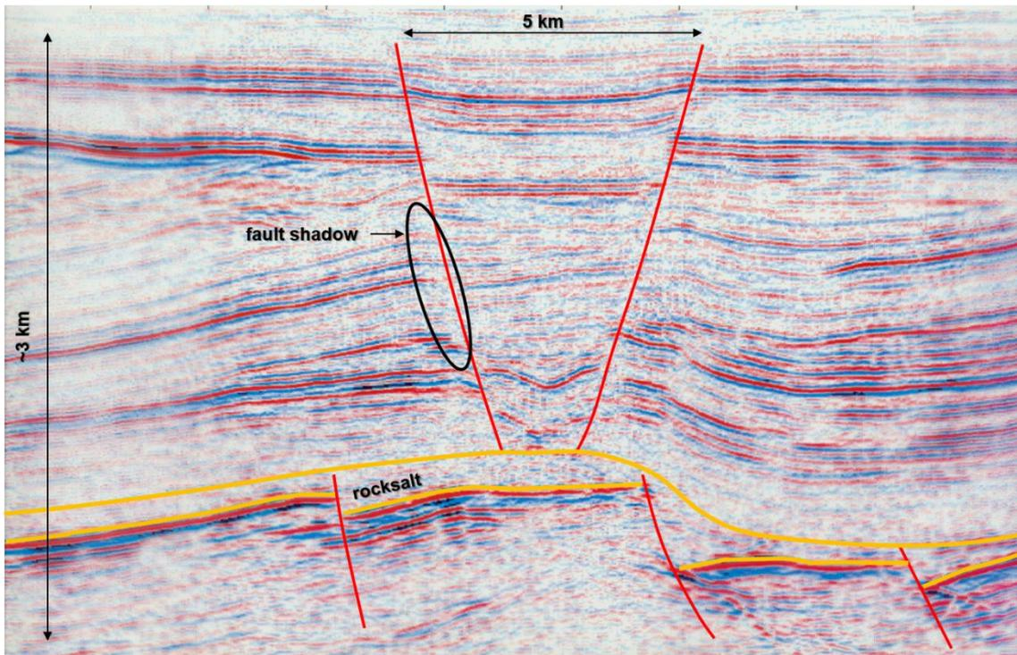
Figure 4-3: Vertical 2D seismic section with interpreted faults (red). The upper faults are blind faults that do not reach the surface. At depth, these faults terminate in a ductile salt layer and can therefore also be classified as detached faults. The faults below the salt layers do not penetrate the salt layer and are classified as buried faults. All faults would be missed in surface outcrops.
