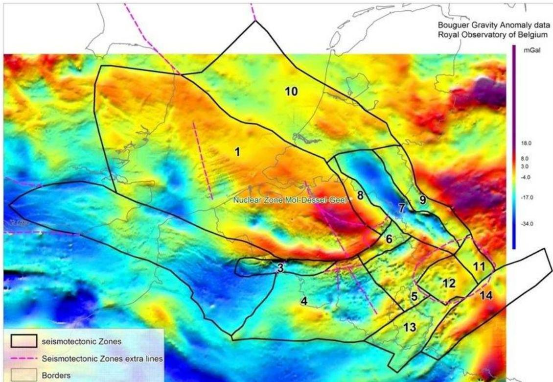
Figure 4-5: Bouguer gravity anomaly data from northern France, Belgium and the southern part of the Netherlands illustrating the delineation of the main seismotectonic zones. Data compiled by Royal Observatory of Belgium. Figure modified after Verbeeck et al., 2009.
