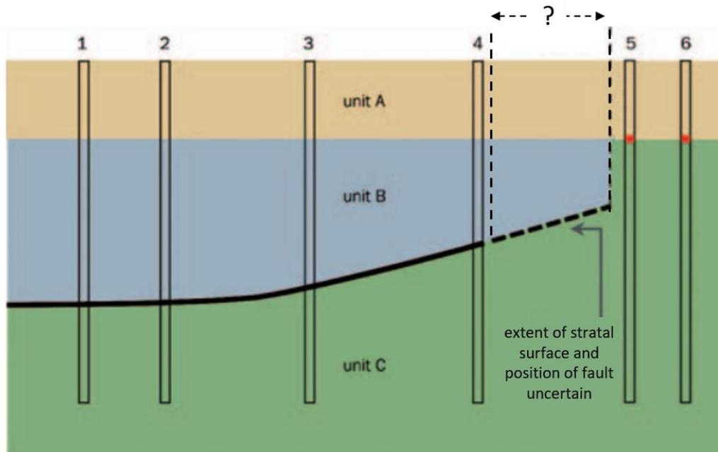
Figure 4-7: Sketch explaining how interpolation of borehole data introduces uncertainties with the proper positioning of faults. Note that an interpretation with pinch-out of unit B (in between wells 4 and 5) is an alternative option that cannot be excluded based on just the borehole data (modified after Gunnink et al., 2013).
