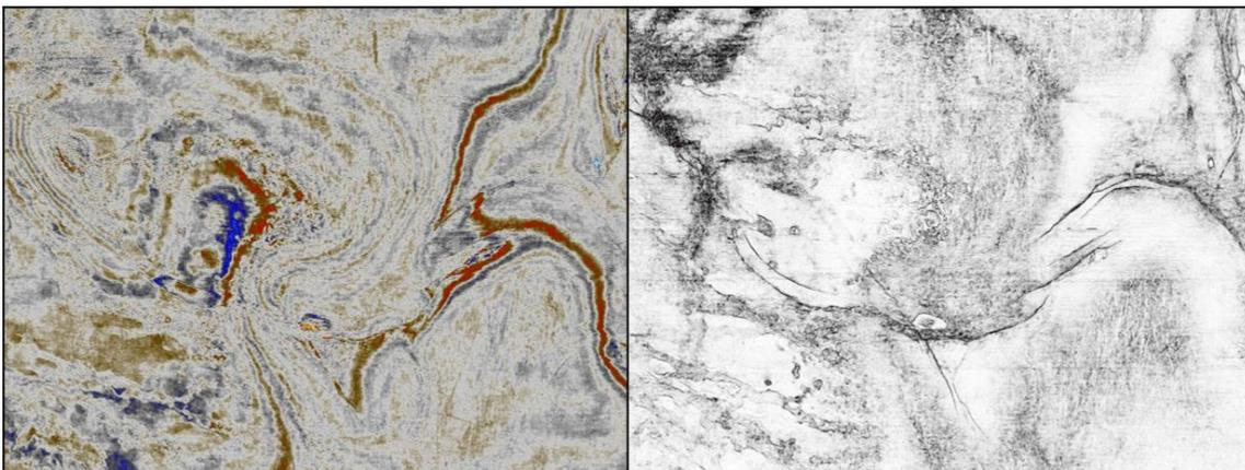
Figure 4-4: Left: horizontal (time-slice) intersection of a seismic 3D amplitude cube. Right: same time slice but now shown with edge-detection attribute that highlights the faults.
