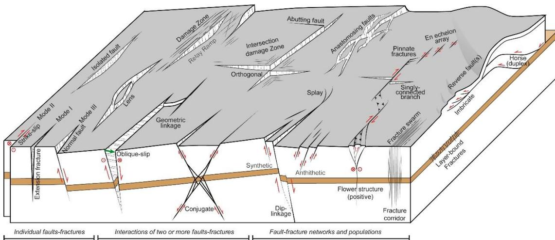
Figure 3-1: Schematic overview of fault types and fault relationships (after Peacock et al., 2016)
