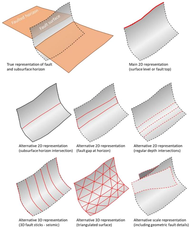
Figure 2-1: Overview of different geometrical definitions of faults
