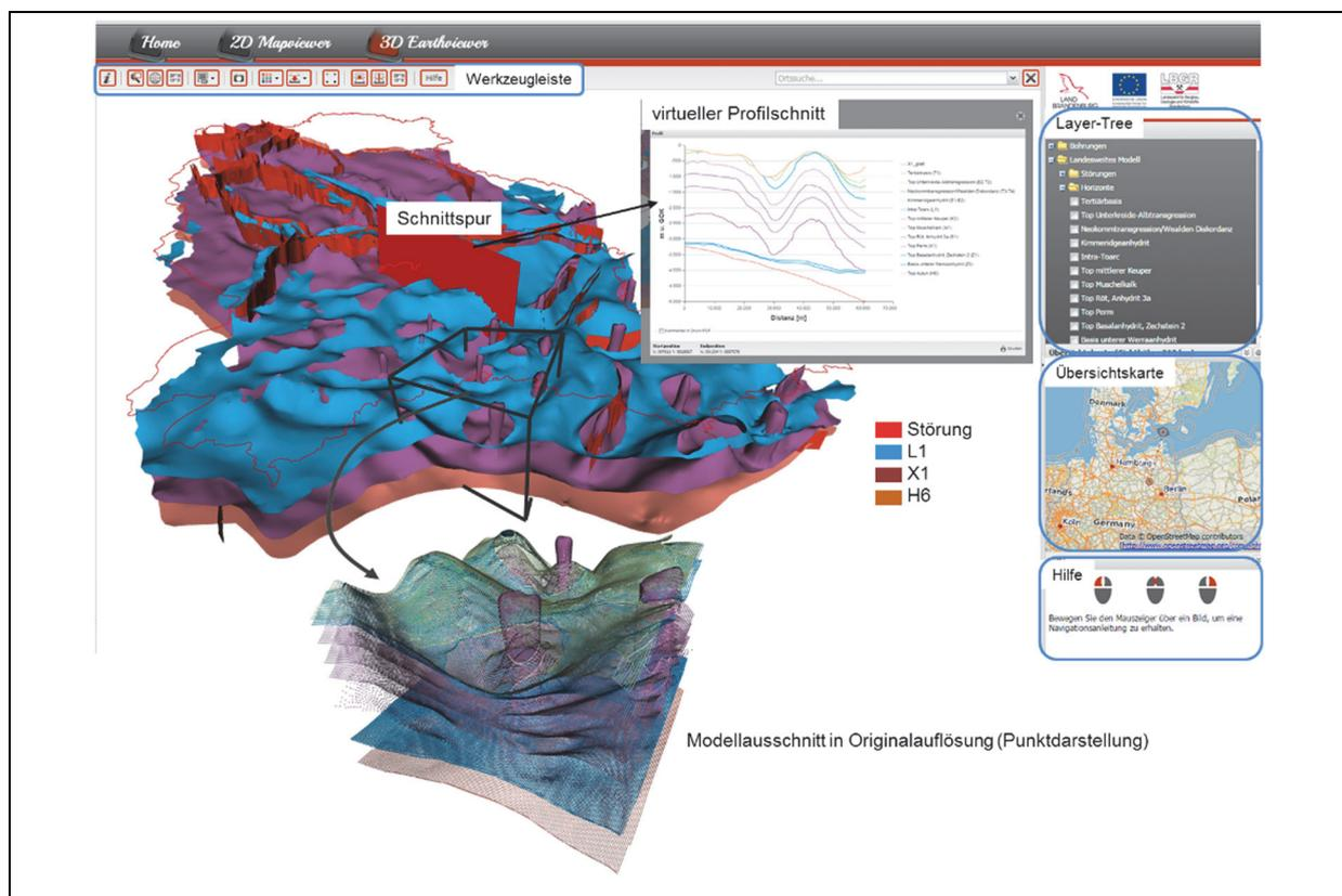
Figure 22: 3D-modell of the subsurface of Brandenburg, web portal: 3D Viewer, representation of some functionalities of the viewer, e.g. creating virtual cross sections and request for model data with original resolution
