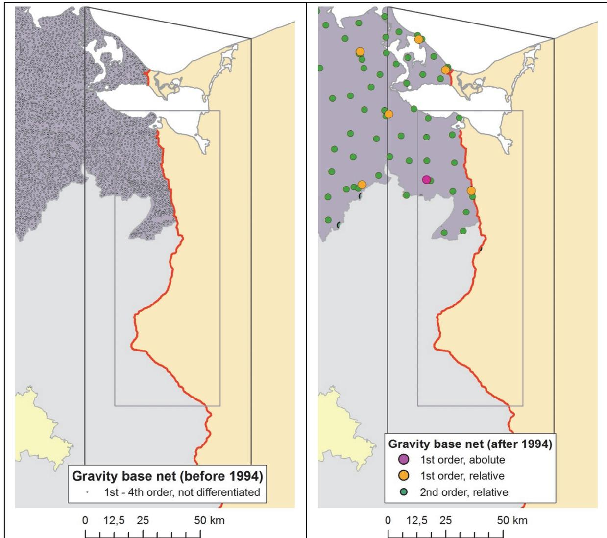
Figure 9: Gravity base network in Eastern Mecklenburg-Western Pomerania. Left: bases 1<sup>st</sup> to 4<sup>th</sup> order 1960-1994 (undifferentiated), right: bases 1994 - now
