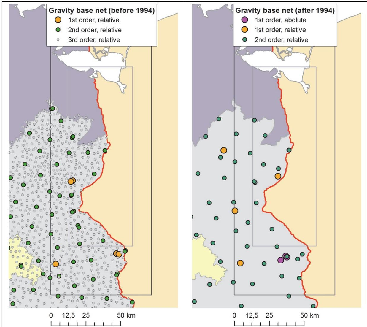
Figure 5: Gravity base network in Brandenburg. Left: bases 1st to 3rd order 1960-1994, right: bases 1994 - now
