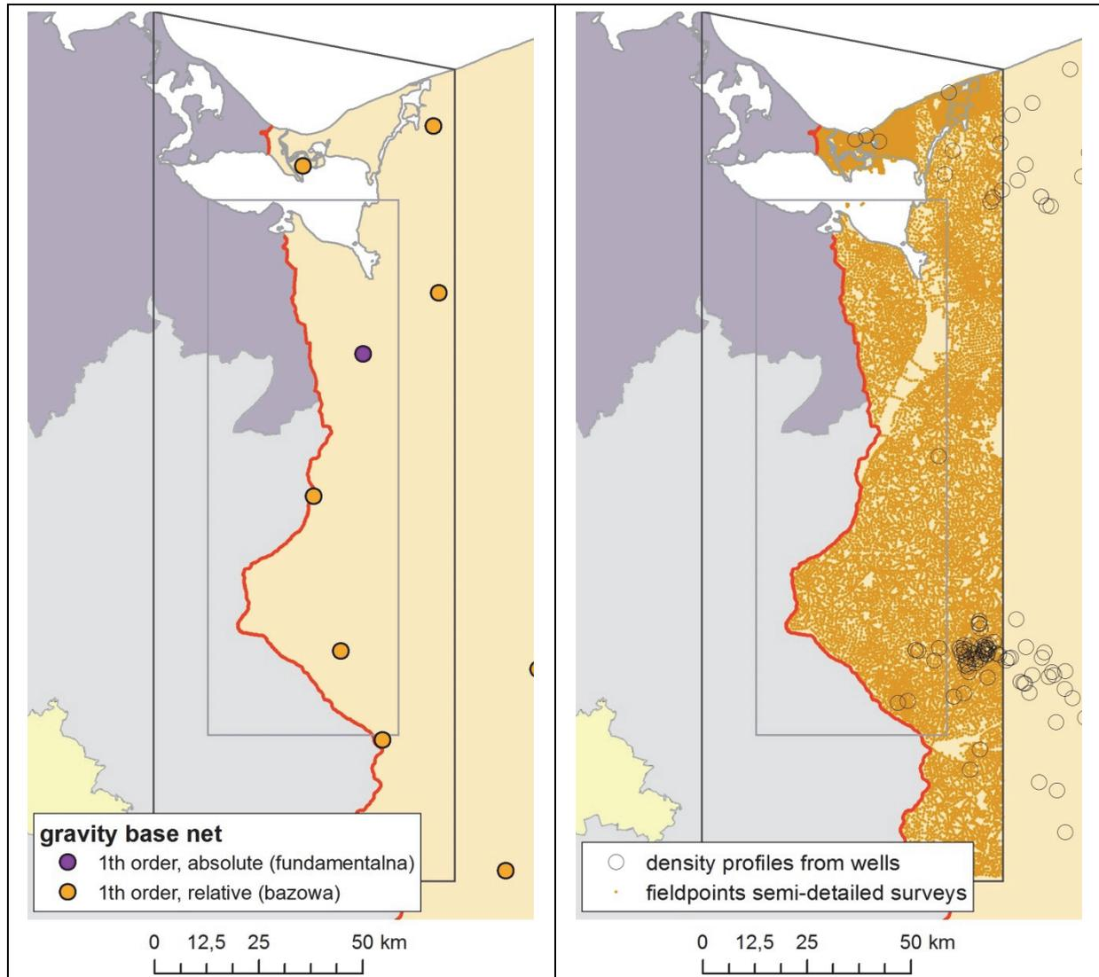
Figure 13: Left: current gravity base network in Poland. Right: seamless semi-detailed gravity measurement points + wells with density profiles
