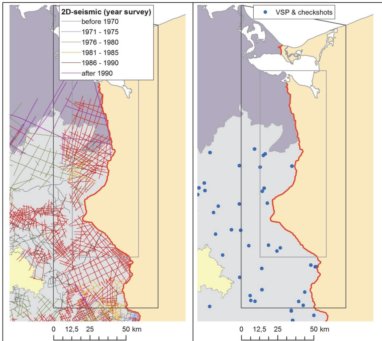
**Figure 4: Seismic investigations in Eastern Brandenburg: left: 2D-profiles area grouped by the year of the survey, right: check-shots and vertical seismic profiles VSP**
