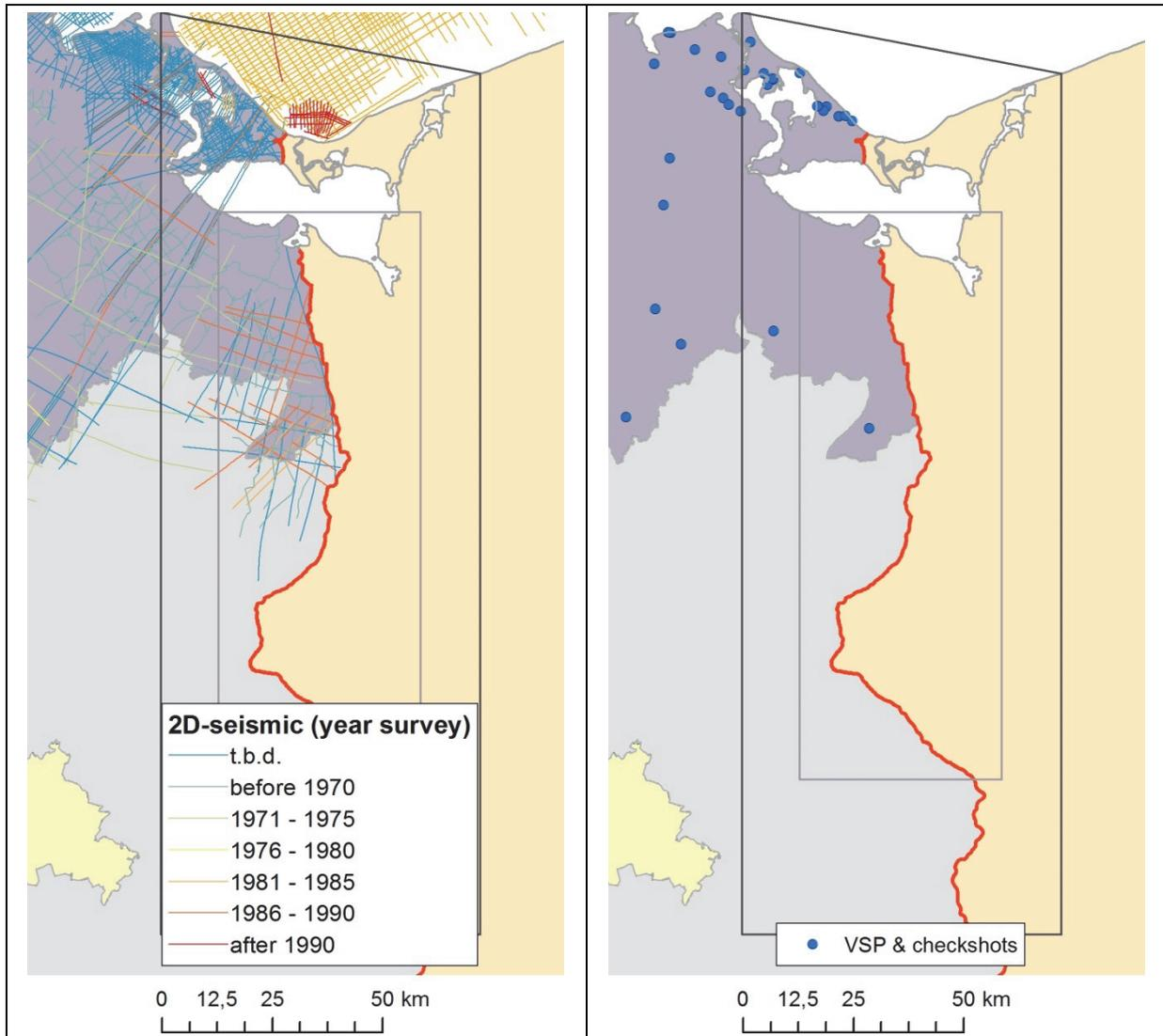
Figure 8: Seismic investigations in Eastern Mecklenburg-Western Pomerania: left: 2D-profiles area grouped by the year of the survey, right: check-shots and vertical seismic profiles VSP
