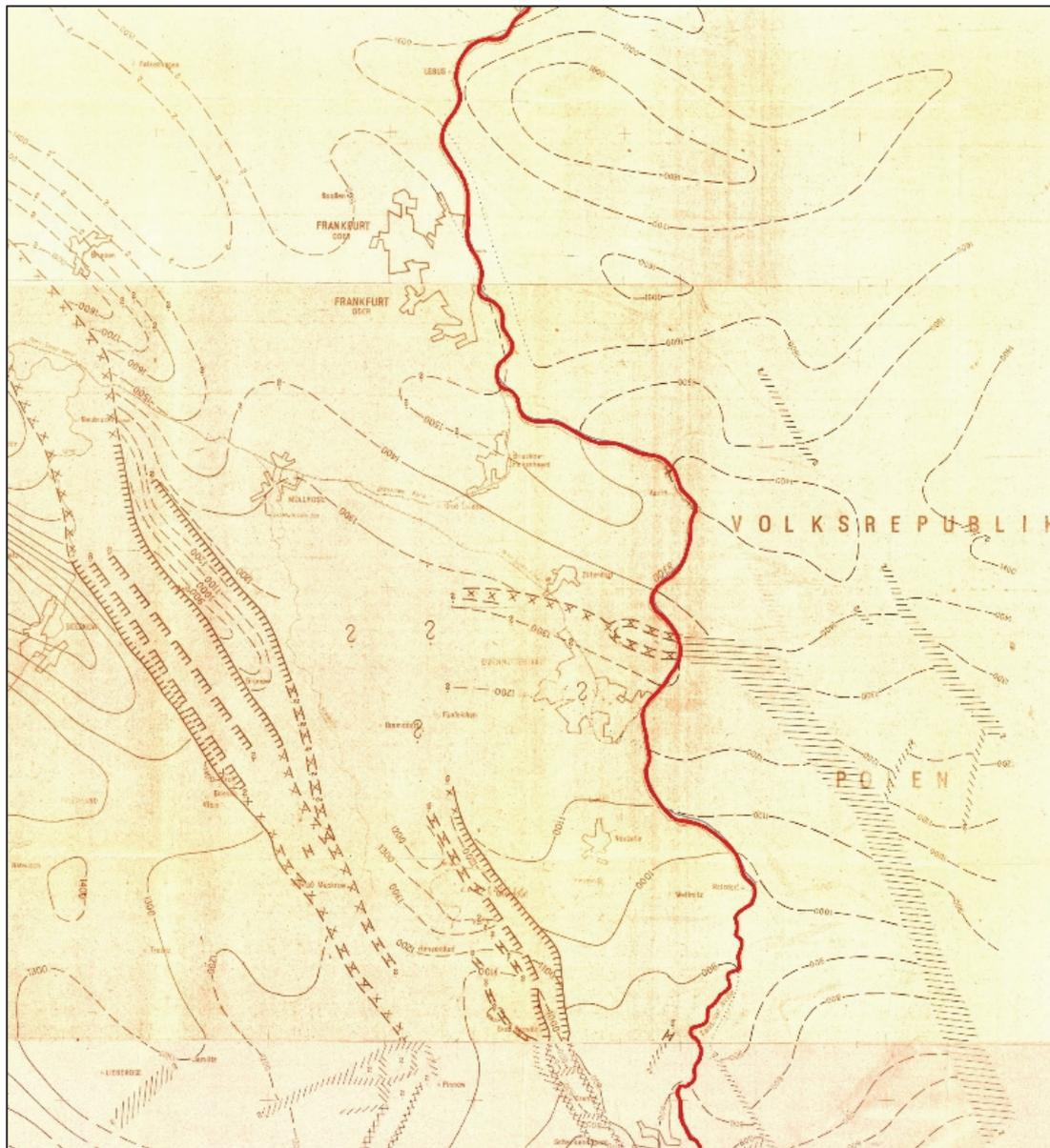
Figure 17: German-Polish harmonization of seismic reflectors 1978-1980, reflector S1, depth contours (detail), scale 1:100.000, border region Brandenburg-Poland (VEB Geophysik Leipzig, Abteilung Seismik 1980)
