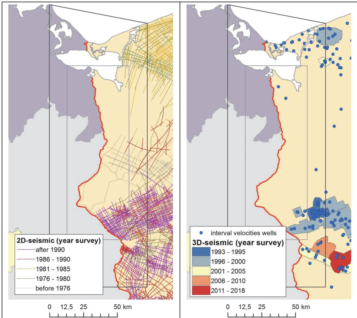
**Figure 12: Seismic investigations in Poland: left: 2D-profiles grouped by the year of the survey, right: 3D surveys grouped by the year of the survey and wells with average velocities.**
