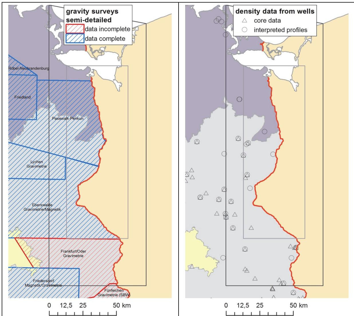
**Figure 6: left: Data availability of semi-detailed gravity surveys in Eastern Brandenburg. Right: wells with petrophysical data (density), core data and interpreted profiles**
