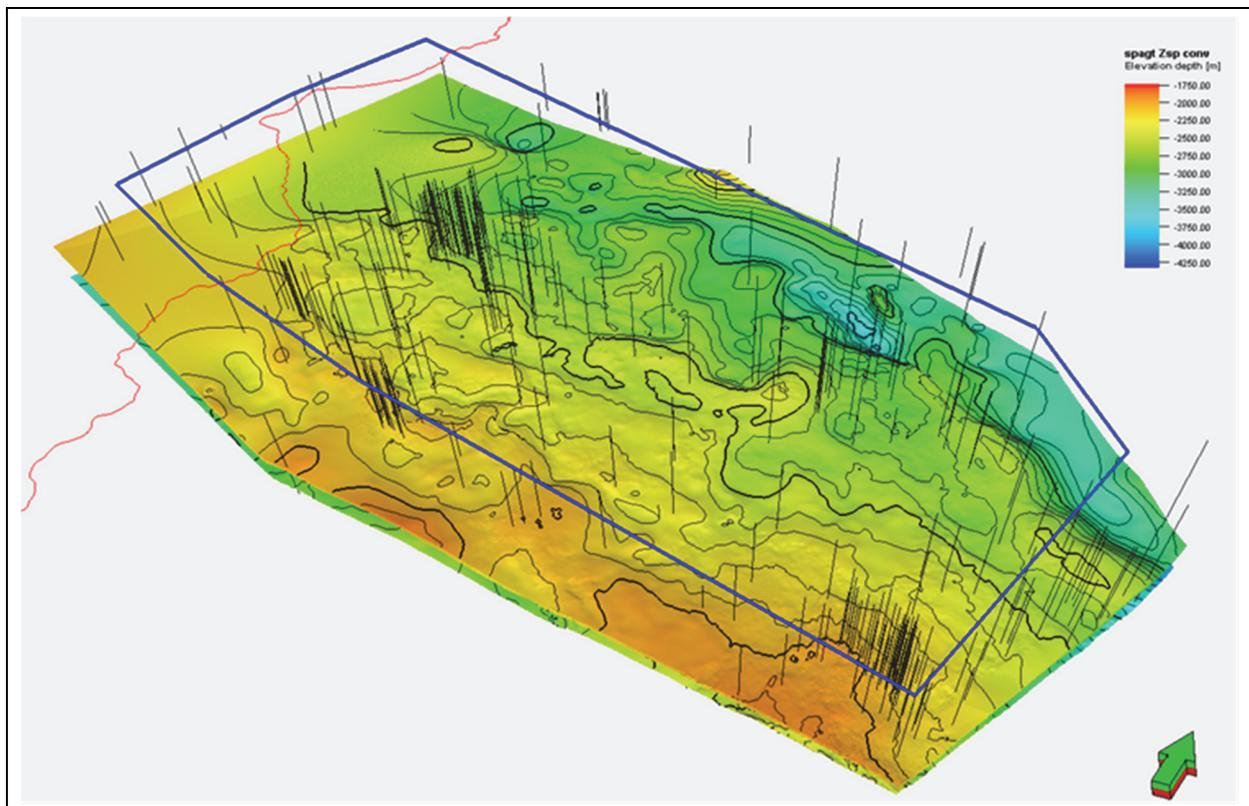
Figure 24: Seismic reflector horizons of Zechstein in 3D geological model of Gorzow Block, Poland (under construction)
