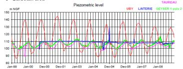
Figure 3.5: Influence of the storage operations on the regional piezometric level (m a.s.l.) A) Temporal evolution of the injected natural gas volume () at Izaute (blue straight line) and at Lussagnet (magenta straight line); B) Temporal evolution of the piezometric level (m) in the nearstorage zone; C) Barbotan area at ≈20 km from the injection wells. (modified from David, 2010)
