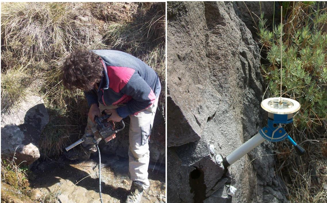
Figure 2.3.11. Paleomagnetic sampling and orientation of samples (cores) with a solar and magnetic compass.
