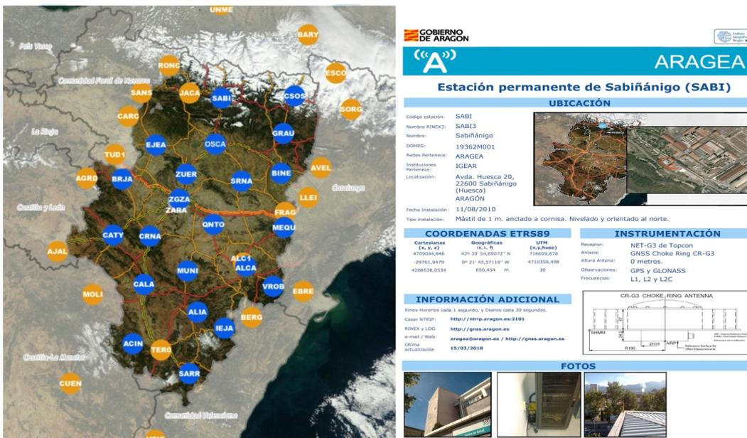
Figure 2.1.19 (next page). Regional ARAGEA network ( <https://gnss.aragon.es/> ) and technical details of one of the Bases (Sabiñánigo) near the 3DGeoEu project target area.
