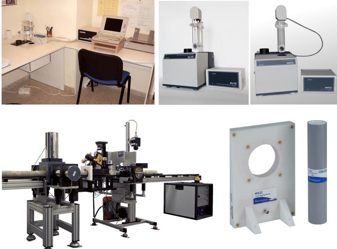
*Figure 2.3.10. Magnetic susceptibility meters for the laboratory. KLY3 at Magnetic fabrics laboratory (U. Zaragoza). The recent KLY-5 and MFK2 models, all of them by AGICO. The Geotek Multi-Sensor Core Logger (MSCL-S) can be equipped with a loop sensor (MS2C, enlarged) and a point sensor (MS2E) that are paired to the Bartington MS3 meter with a measuring range of 26 SI.*
