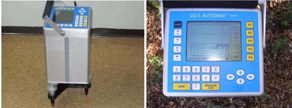
Figure 2.1.6. Left) Scintrex CG5 on its tripod. Right) view of the CG5 display.
