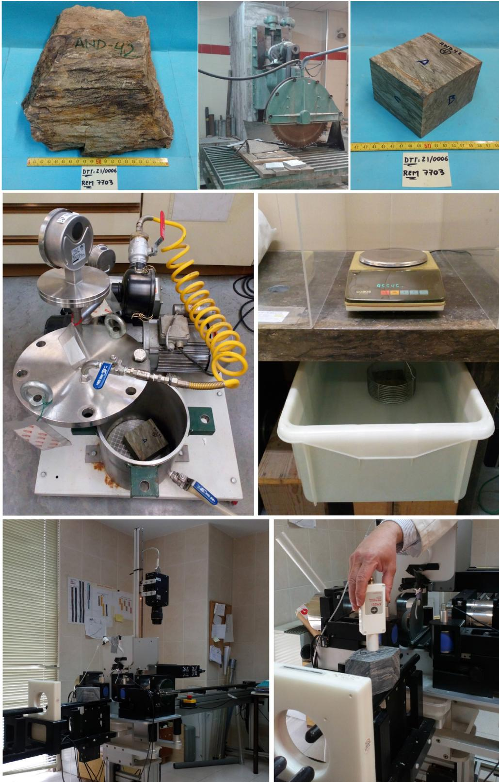
Figure 2.3.8 (cont). Cutting hand samples and pressurized chamber at IGME laboratories (Madrid).
