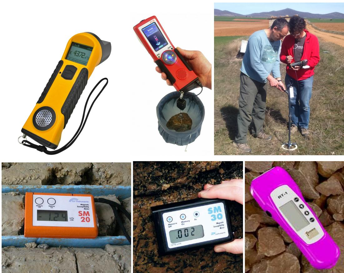
Figure 2.3.5. Some portable magnetic susceptibility meters available in the market. From up left to downright: KT10 and KT20 by Terraplus (this last one with the density upgrade), SM20 by GF Instruments, SM30 by ZH Instruments, RT-1 (former by Fugro and by CorMaGeo) now by Bartington and the MS3 multi sensor susceptibility unit with a MS2D surface coil by Bartington.
