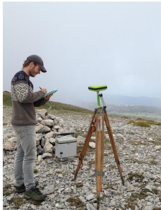
Figure 2.1.5. Left) the ZLS Burris gravimeter. Right) Measure taken with a Burris gravimeter at Tozal de Guara summit (2008 m) in the External Sierras (Southern Pyrenees)-DR3AM project.
