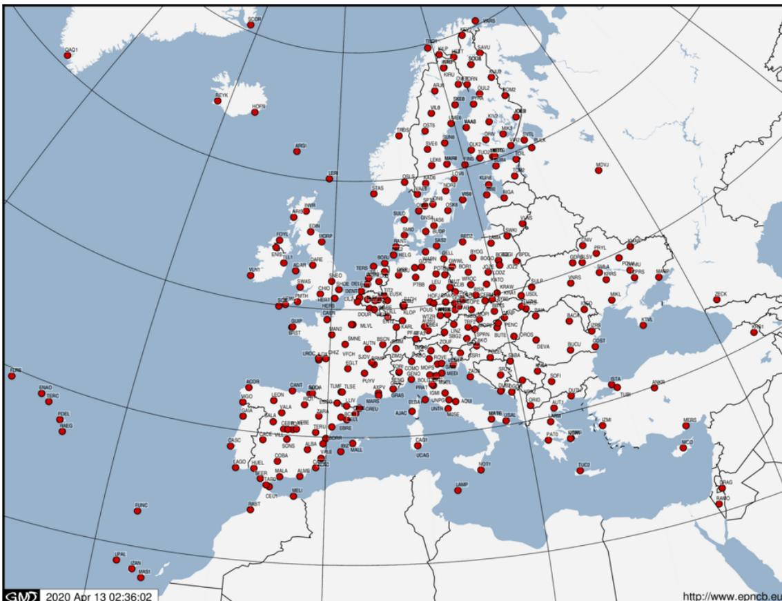
Figure 2.1.17. EUREF Permanent GNSS Network. Example of location of stations providing real-time data (source <http://epncb.oma.be/>).
