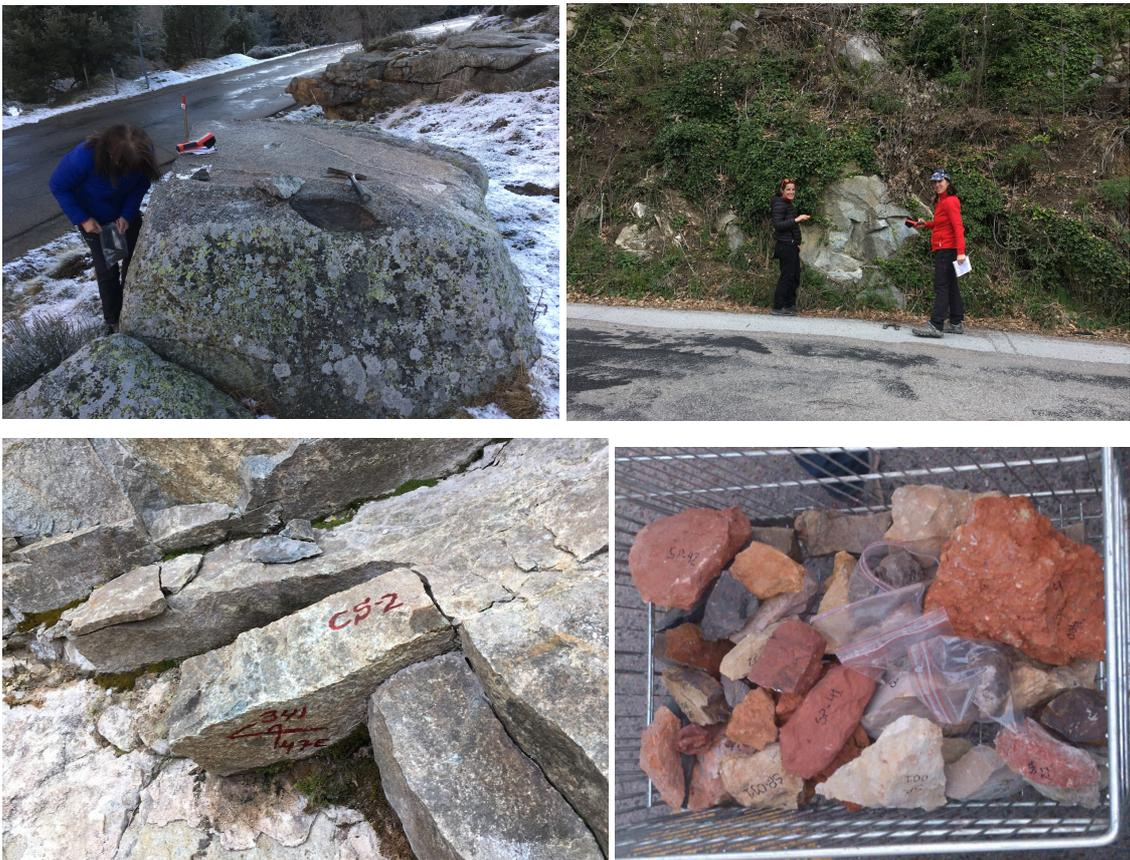
Figure 2.3.4. Petrophysical hand sampling in the outcrop. All pictures; sampling igneous rocks in the Pyrenees, except for the bottom right one; hand samples from the Iberian Range (Pueyo et al., 2016a).
