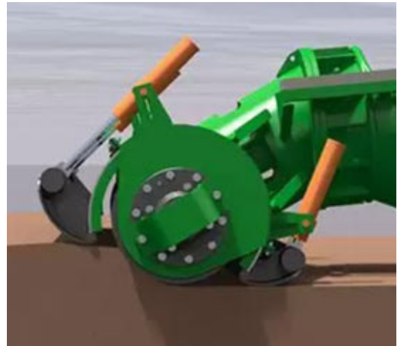
Figure 1: Example of auger dredger with a retractable visor which closes around the auger when dredging to prevent particles from spreading. Source: www.dredgeyard.com
