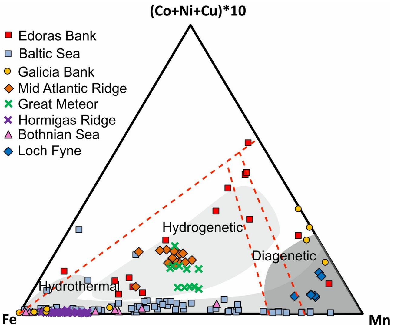
**Figure 6.** Relationship among Co+Ni+Cu, Fe and Mn, for polymetallic nodules registered in MINDeSEA database (ternary diagram from Bonatti *et al.*, 1972).
