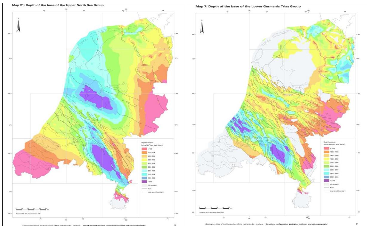
Figure 13: Depth maps of the base of the Upper North Sea Group and the base of the Lower Germanic Trias Group which clearly show that a few faults are crossing the German-Dutch border in the pilot area
