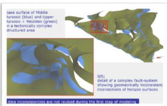
Figure 4: GTA3D - example of data inconsistencies; intersection of base surface of Middle Jurassic (blue) and base surface of Upper Jurassic+Wealden (green) (Helms 2018, unpublished).
