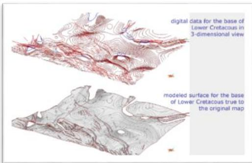
Figure 3: GTA3D – example of the modeling workflow of the Lower Cretaceous horizon, based on digitized maps (Bombien et al. 2012).
