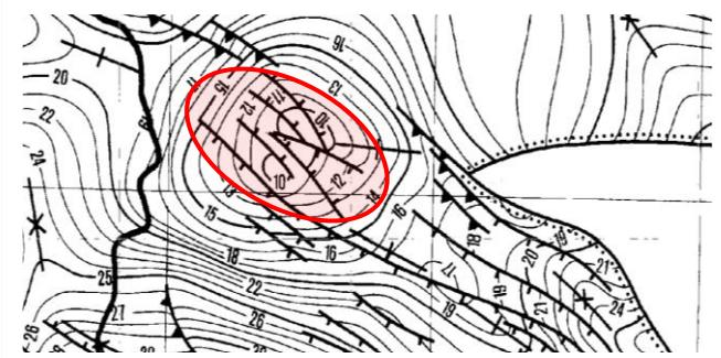
Figure 9: Detail of GTA map "base Lower Jurassic" showing fault traces and additional information (e.g., dip angle and dip direction and the fault shows a horizontal and vertical displacement) (e.g., red circle) of faults; modified after (Baldschuhn et al. 2001).
