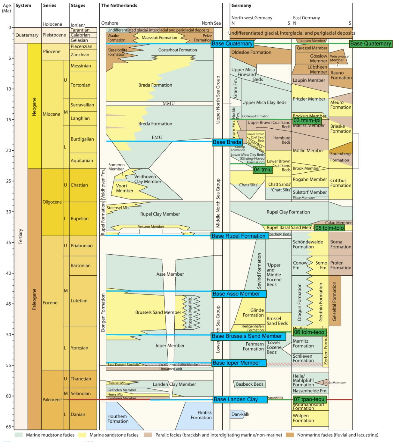
Figure 10: Tectonostratigraphic Chart for Cenozoic (modified after (Doornenbal and Stevenson, 2010)). The red line is the seismically mapped near base Cenozoic in the SPBA-project. Blue lines show the seismically mapped horizons of DGM-NNL (Rupel Formation consists of modeled layers: Rupel Clay and Vessem Member) and the green lines show the seismically mapped horizons of GTA3D.
