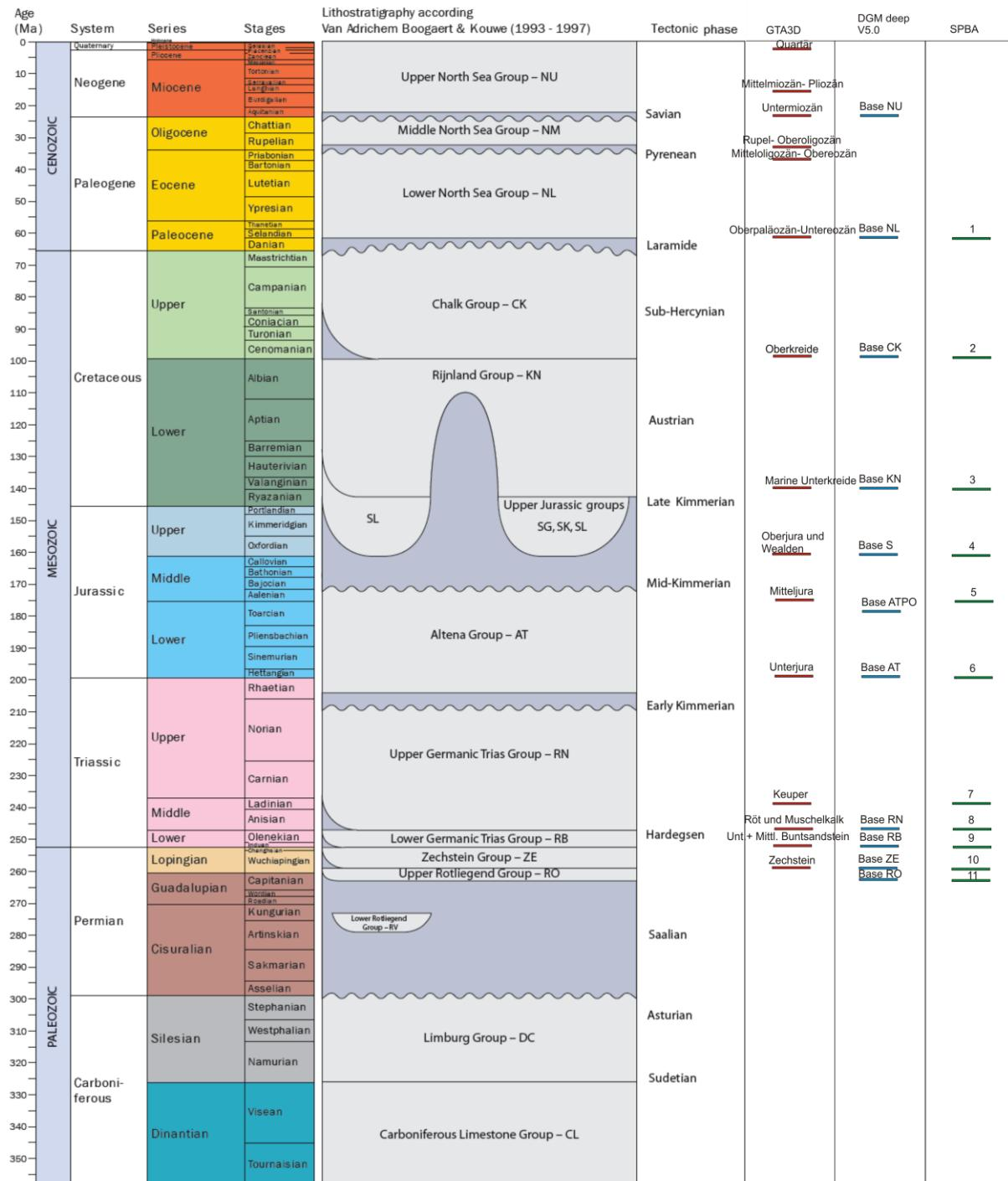
Figure 11: correlation of modelled layers for GTA3D (red lines), DGM deep (blue lines) and SPBA ( green lines) with names of the modeled horizons(modified after (Kombrink et al., 2012))
