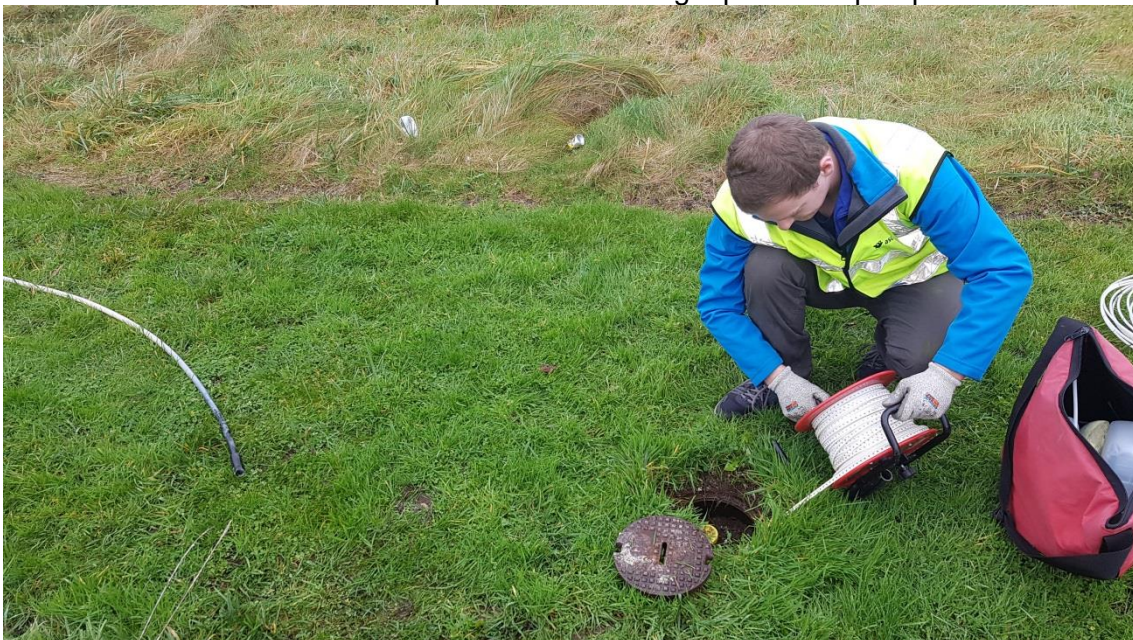
Figure 25. Using the dip-metre to collect groundwater level and temperature measurements from a borehole.
